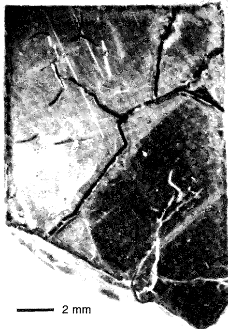
Fig. 8 Microcracks in a Te-doped ingot grown at 9 g.
